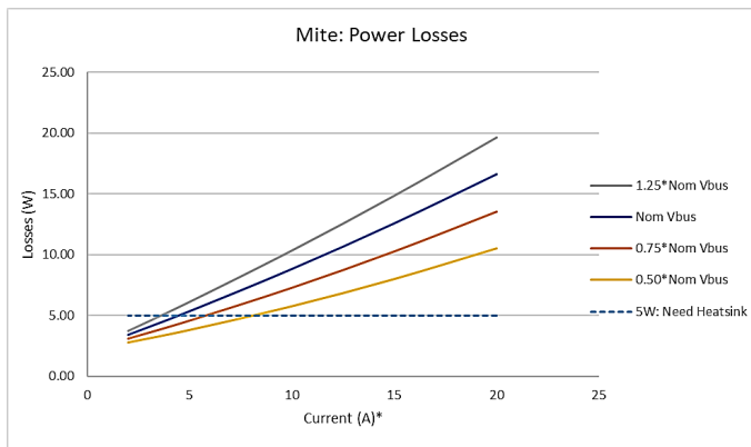
M20A028VPS Power Loss Curve
