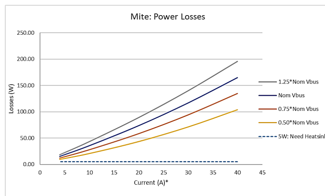
M40A048VPD Power Loss Curve
