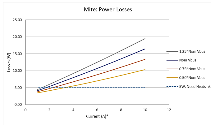
M10A028VPD Power Loss Curve
