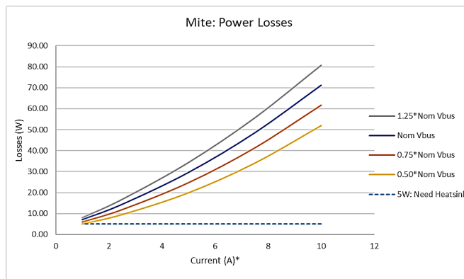
M10A170VPD Power Loss Curve
