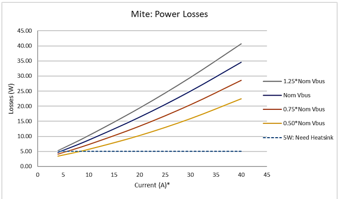
M40A028VPS Power Loss Curve
