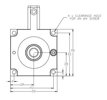
ACTUATOR BODY T-SLOT MOUNTING FEATURES
